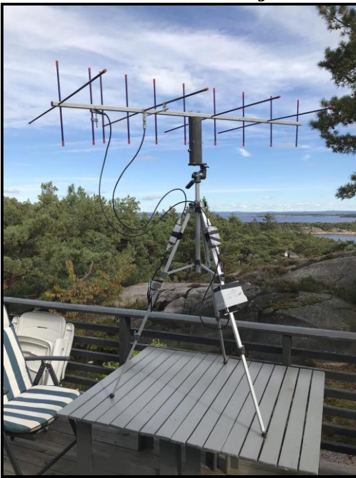
2m and 70cm antennas on tripod used by JW7XK
